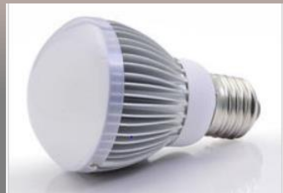
A modern retrofit LED lamp with "bulb" shape, complete with aluminium heatsink, a light diffusing dome and E27 screw base, using a built-in power supply working on mains voltage
